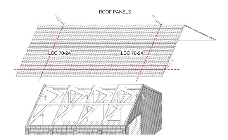
Glue LCC 70-24 together to create two roof tile panels.
