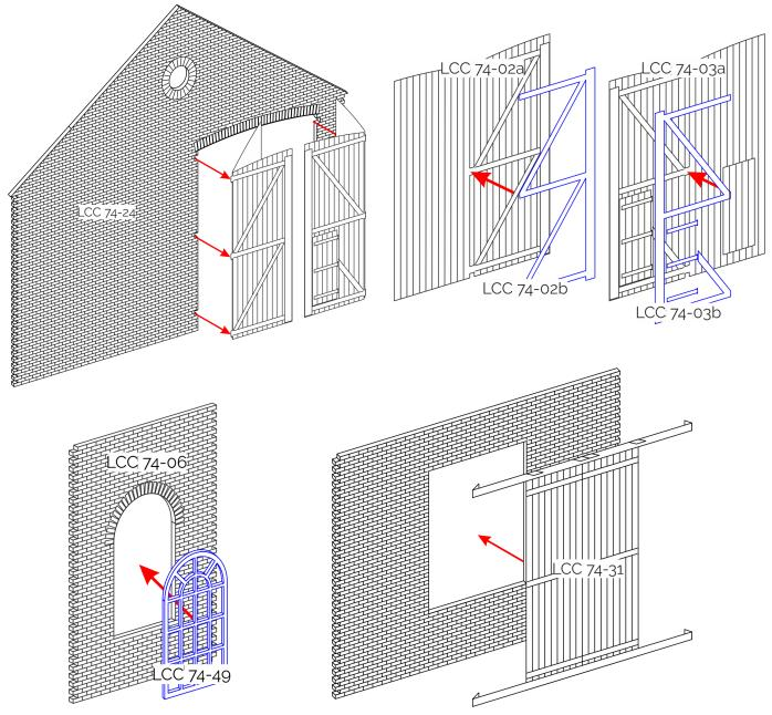
After the main building was assembled and painted, paint and pre assemble the fittings.
