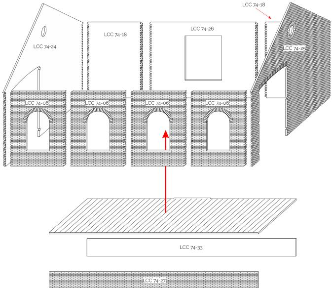
Build the structure of the goods shed first before tackling the buttresses and corners. Start by joining the walls made up of LCC 74-06, LCC 74-18, and LCC 74-26. Leave to dry. Then join the walls with the gate panels LCC 74-24 and LCC 74-25. Make sure the gate opening is on the window side.
