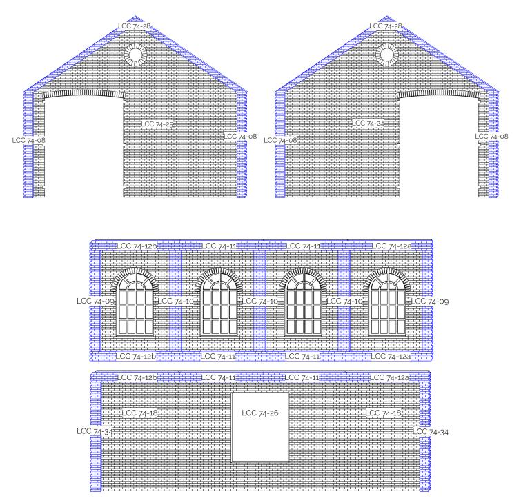
Start with the corners (LCC 74-08, LCC 74-09, and LCC 74-34). Make sure to orient them in the same orientation as in the spruce (part number up). On gate elevations (LCC 74-24 and LCC 74-25) they should run from the bottom and meet with LCC 74-28. On the elevation with windows they should have equal space on the top and bottom for LCC 74-12. On the elevation with the gate they should run from the bottom and only have the gap on the top.
