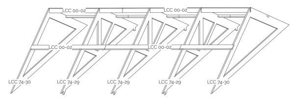
Diagram above shows the roof truss structure as if it was assembled outside of the engine shed. We recommend not to assemble it outside of the shell unless a removable roof is required.
