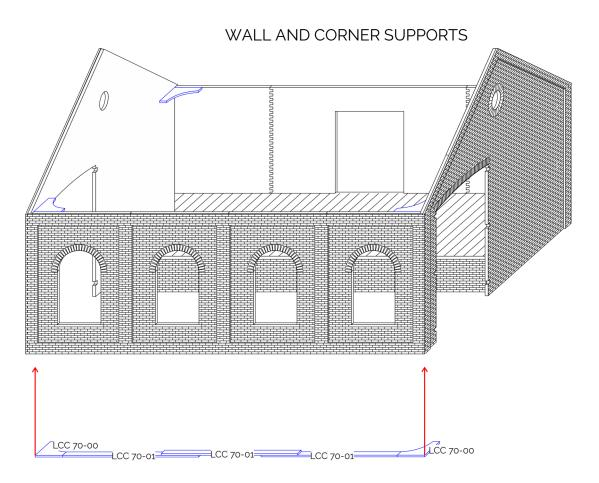
Use parts from LCC 70-00 and LCC 70-01 to stiffen the walls and corners.. They are optional parts and can be omitted if desired.
