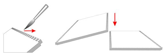
Recommended way of gluing parts together is to apply PVA glue to the interlocking bricks working from back of the part to the front. This ensures there will be no glue overflow on the front, visible side. Then lay the part without glue on flat surface laying on its front (engraved side). Press the part with glue onto the part without glue. Gently push parts together from sides to close the gap.
