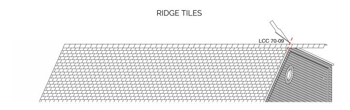
The ridge tiles (LCC 70-09) need to be folded in half and then glued over the seam between the two roof sides. Score the fold line with a hobby knife for easier folding.
